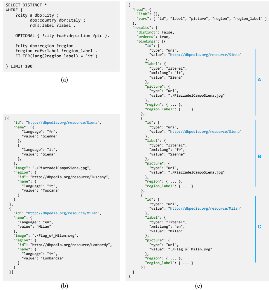
Fig. 1. A SPARQL query (a) extracting a list of Italian cities with picture, label and belonging region, of which the URI and the Italian name are also requested. In the standard output of the endpoint (c), the city of Sienna is represented by both object A and B, while the transformed output (b) offers a more compact structure.
