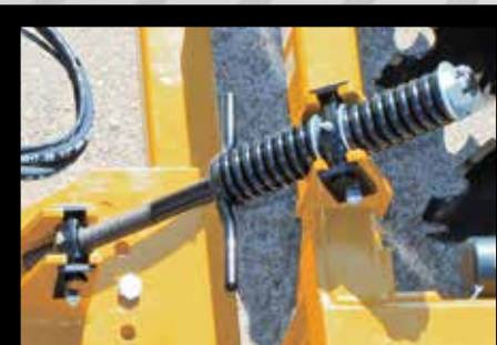
Right: Spring leveling system absorbs shock when the disc is pulled over uneven terrain.
