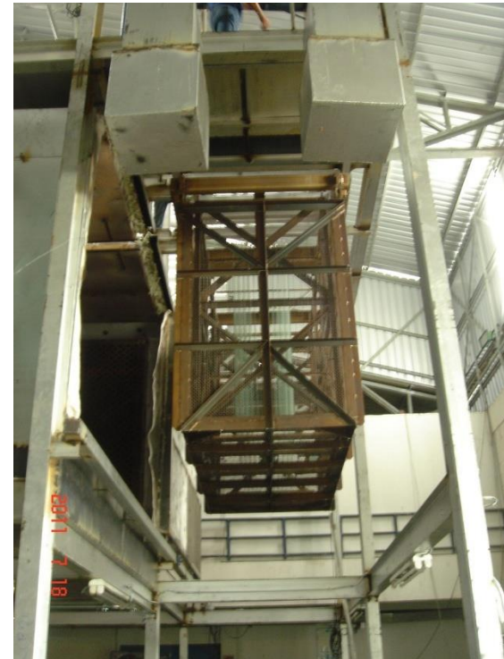
Lift up Float Glass into Heating Zone
