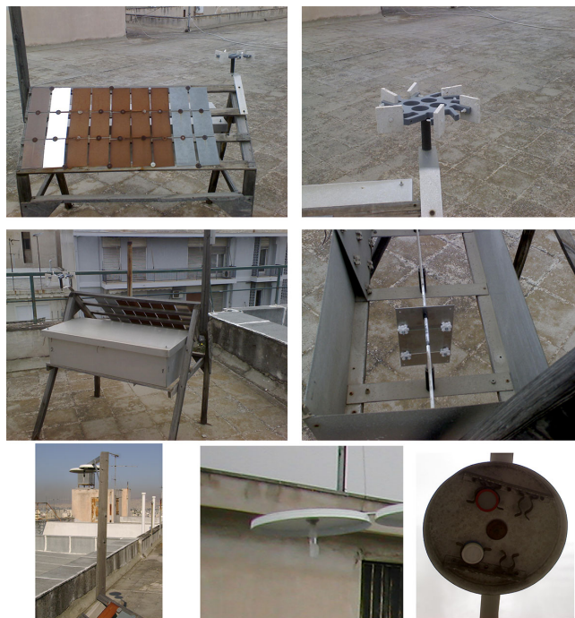
Figure 1. The exposure site in the centre of Athens (Greece). The top panel shows the carousel (on the right) and the main rack (on the left) with the material specimens. They consisted of an inclined plane and an aluminium box with open bottom (middle panel). The middle panel shows aluminium box (on the left) and the glass specimens inside the aluminium box (on the right). The bottom panel shows the diffusive passive samplers for the surface air pollutants measurements and the passive particle collector under the rain shield.
