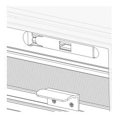
Leave a space of around 10mm between the front of the blind and the edge of the recess, so that there's space to fit the pelmet on the front later. Ensure that there is a gap of at least 50mm between the back of the blind and the window frame.
