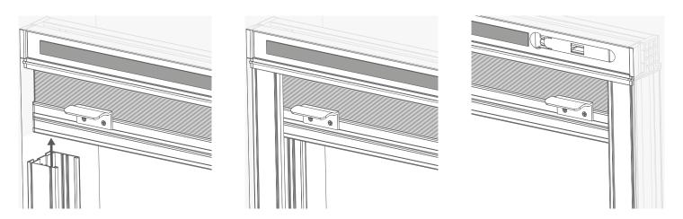
Push the channel upwards as you straighten it up, slotting it up onto the cap on the end of the blind's headrail, so that the channel sits flush against the underside of the headrail. Do the same for both side channels.
