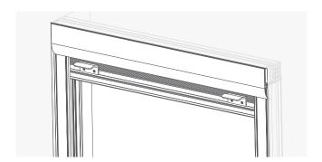
Finally, attach the pelmet to finish. The pelmet simply attaches with magnets, just line up the magnets on the back of the pelmet with the strip on the front of the blind's headrail and press into place.
