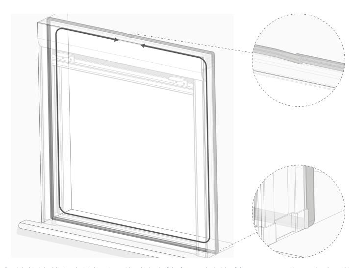
Reach behind the blind and stick the strip to either the back of the frame or the inside of the recess - try to make sure that the seal is tight to both the back of the blind and the inside surfaces of the recess, even at the corners. Ideally the two ends of the strip should meet together around the centre at the top of the blind. Use a pair of scissors to trim away any excess, leaving a small overlap.
