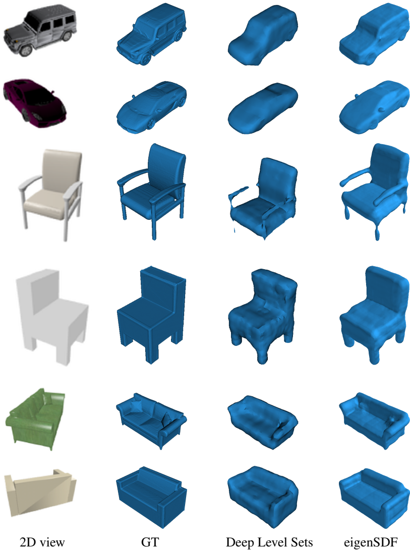
Figure 5: We compare reconstructions of eigenSDF and the CNN decoder based Deep Level Sets [22] without limiting eigenSDF to low resolution as it allows us to operate at a higher resolution and generally produces more locally coherent results.
