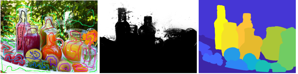
Figure 4: Illustrating the use of model-based segmentation methods: The user scribbles different objects to be segmented (left) from which a unary data term f is generated, e.g. by approaches like [49] or a pointwise neural network. As the unaries are insufficient for a good segmentation (illustrated by the fact that a thresholding of the unaries shown in the middle does not segment the background well), the proposed framework offers an efficient approach to obtain accurate segmentations as shown on the right.
