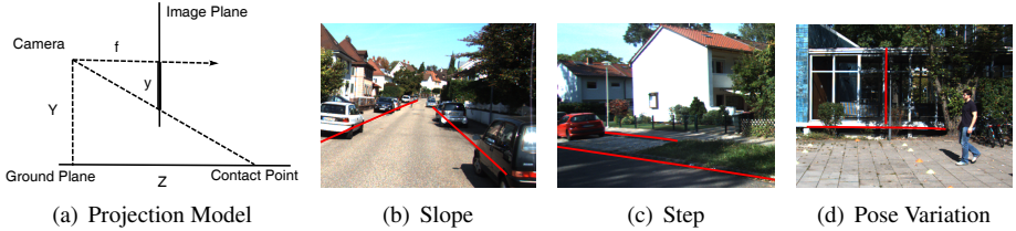
Figure 1: (a) Illustration of depth estimation from the image coordinate of the object. (b)-(d) Examples of real situations. We highlight some representative lines (red) that provide information about slope, step and camera pose variation respectively.
