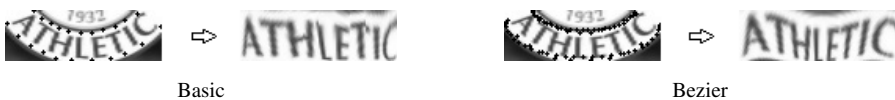
Figure 6: Illustration of the effect of Bezier curve-based dense sampling of slicing grid points on the rectification result. The crosses in the original image indicate the control points of the slicing grid.
