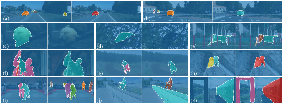
Figure 5: Example of Raptor failure cases. The left of the image pairs shows GT and the right the estimated segmentation. The most common failure cases are due to a small apparent motion (a,b,c). Others problems include: obstacles (d,e), merging moving object instances (f,g,h), false-positive detection for semantically meaningful objects (i) and optical flow failure (j). Sometimes, the GT is incomplete and we discover missing objects (k).
