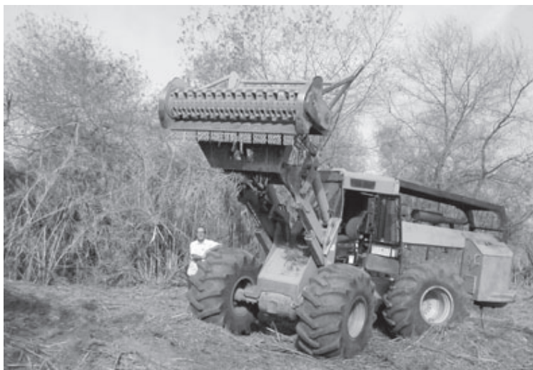
Figure 2 (top). Ammbusher rotary mower is effective at clearing Arundo between closely spaced trees and on steep slopes. Figure 3 (bottom). Hydro Ax hammer-flail mower cuts and mulches as much as 1 ac/day of dense Arundo .
