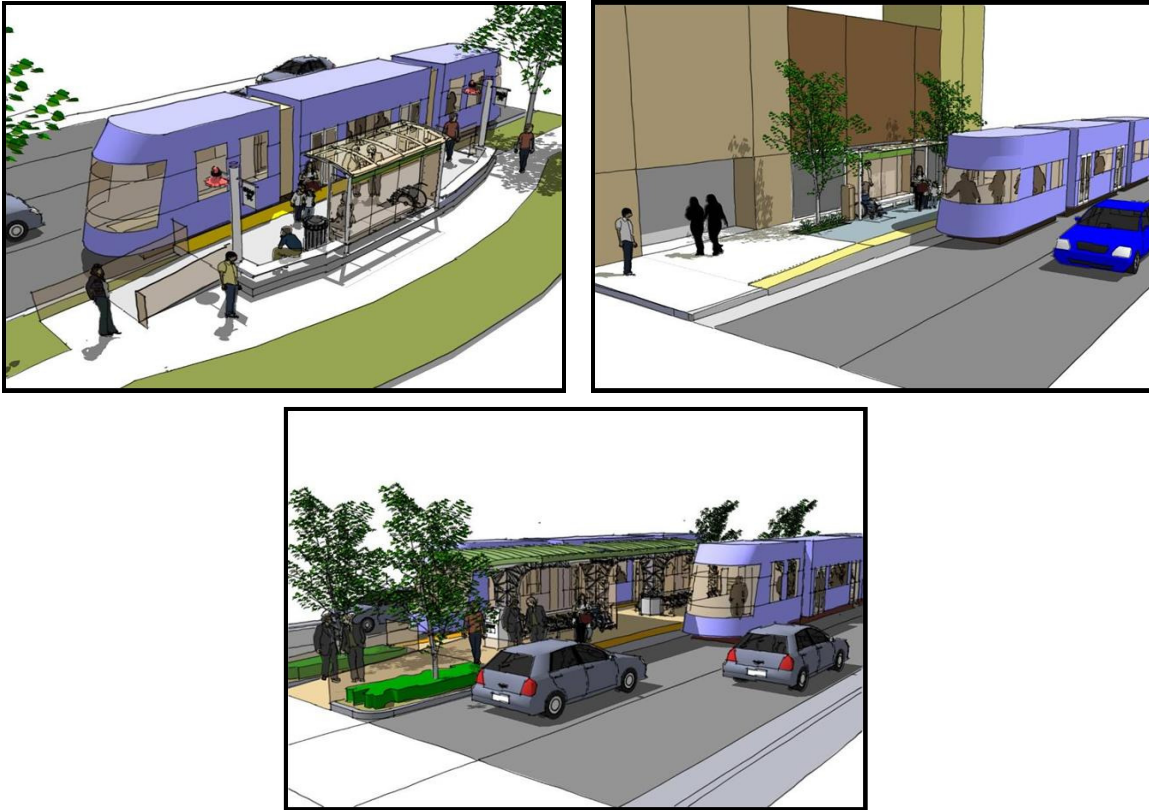
Exhibit 5: Standard Side Platform, Typical Side (Narrow) Platform, and Typical Median (Center) Platform
