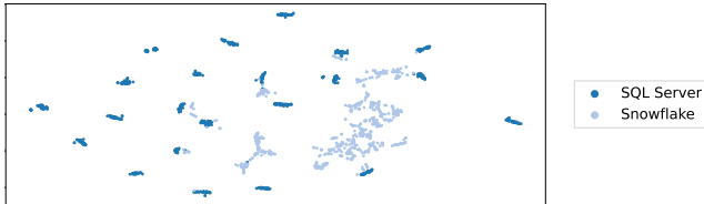
Figure 5: t-SNE visualization on TPC-H (SF10) for Snowflake and SQL Server ( p = 20, i = 2000 ), clustered on operator shares.
