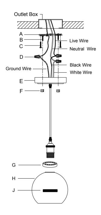
In view of thermal expansion and contraction, avoid securing the glass shade too tight when screwing the socket ring into the lamp holder, or you will break the glass shade.
