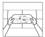
1. Stick self-adhesive template on to duct (a template is provided with each door)
