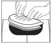
3. Install door by unscrewing the 4. Turn straight and pull out slighlty hand knobs until thread is level to align. Then tighten knobs. with top of bolt. Using both hands place the door in the hole at an angle.
