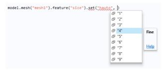
COMSOL Multiphysics and its add-on modules contain thousands of physics features that you can learn about by using, for example, **Record Code**, **Save as** > **Model File for Java**, and code completion. The figure below shows code completion for a particular feature in the **Electric Currents** interface.
