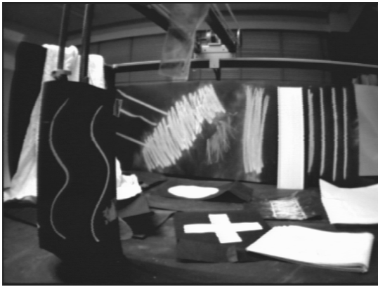
Figure 8.5: A view of the gantry robot taken directly from the panning camera head. The gantry, visible on the left of the image, has had a large dark cylinder of paper with vertical white wavy lines wrapped around it.
