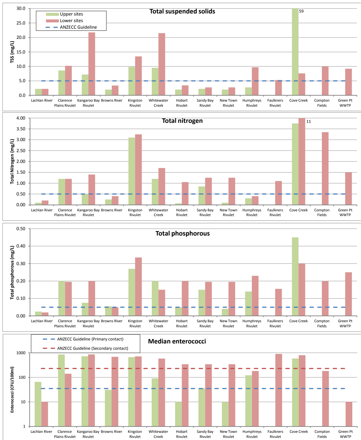
Figure 4.12 Monitoring results for Derwent rivulet and stormwater monitoring program (2011–12) showing median values of TSS, TN, TP and enterococci at upper and lower sites
