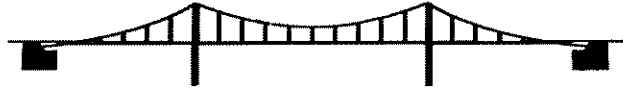
Figure 3: Suspension Bridge (Source: U.S. Department of Transportation, Federal Highway Administration, Safety Inspection of In-Service Bridges, Participant Notebook, Volume II, Publication No. FHWA-HI-91-021 . Washington, D.C. Federal Highway Administration, 1992).
