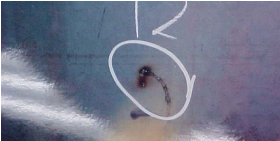
Example of an arc strike
