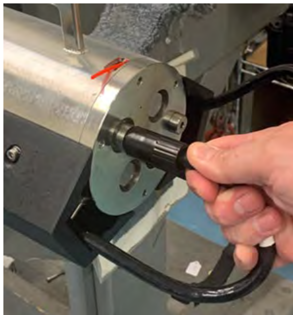
Figure 7-2: Aft Endcap Cable Disconnection
