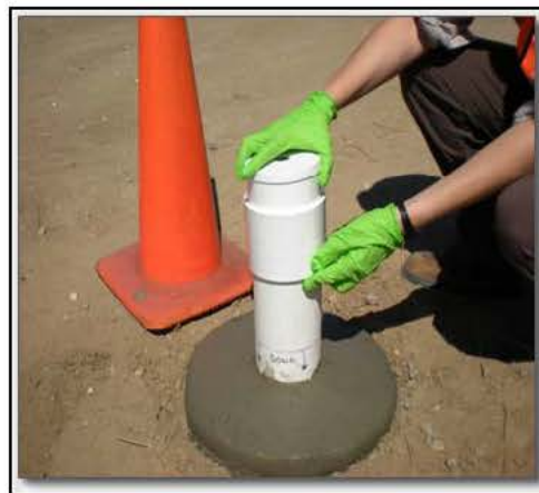
CO 2 trap developed by Colorado State University to measure LNAPL loss rates in the field 121
