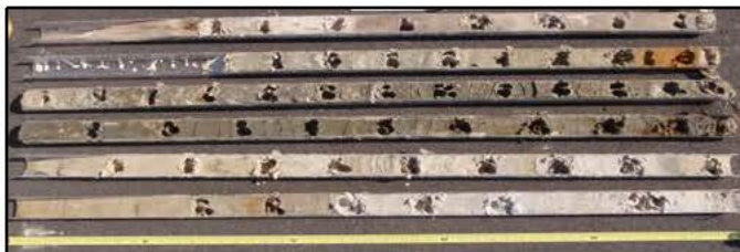
Example of high-resolution sub-sampling of soil cores for assessing attenuation in low-k zones
