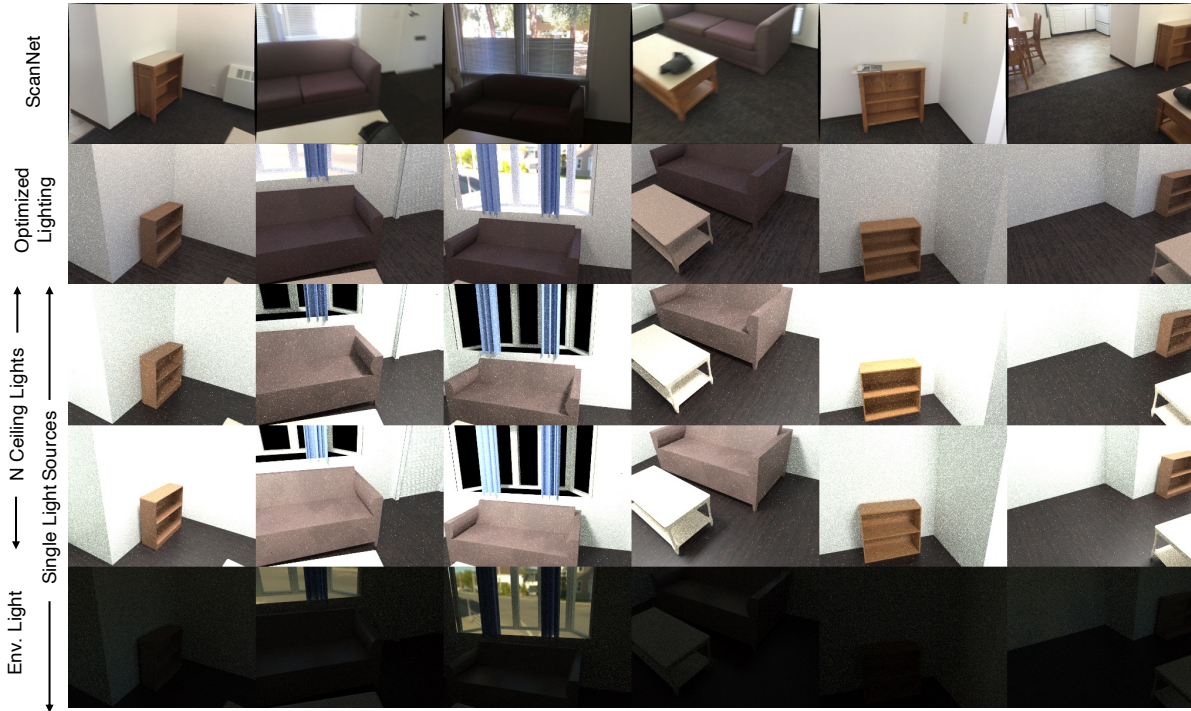
Figure 3.6. Example of lighting optimization result using N = 2 ceiling lights and one environment map lighting. The optimized lighting is close to original ScanNet images.
