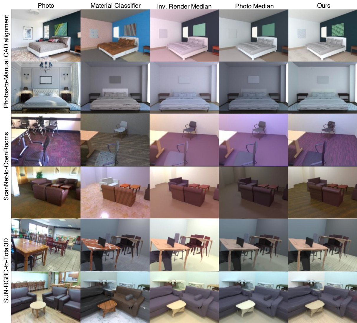
Figure 3.13. Qualitative comparison 2 with baselines on various datasets, where our method generates high-quality materials with spatially-varying patterns that better match the input photograph.
