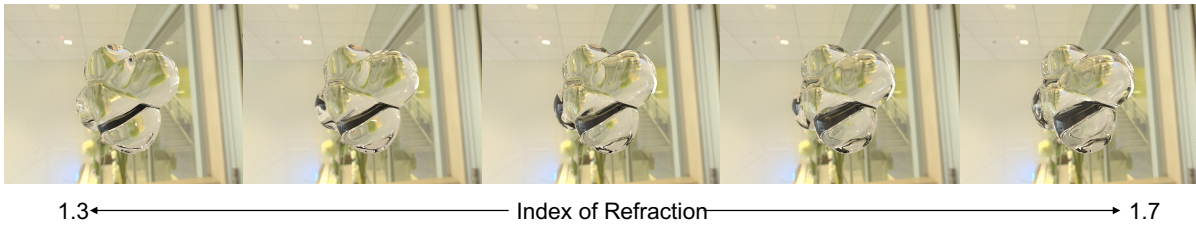
Figure 5.19. Appearance changes for same shape geometry under various index of refraction (IoRs). IoRs range from 1.3 to 1.7.
