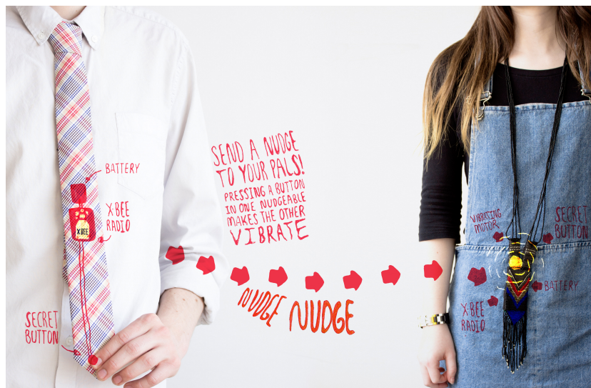
Figure 2.12: An Illustration demonstrating how the Nudgeables can work in the social space
