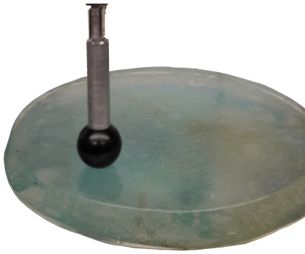
(a) Real world view of a silicone phantom palpation experiment. During palpation a load is applied to the phantom using the black palpation tool, which presses into the phantom surface.
