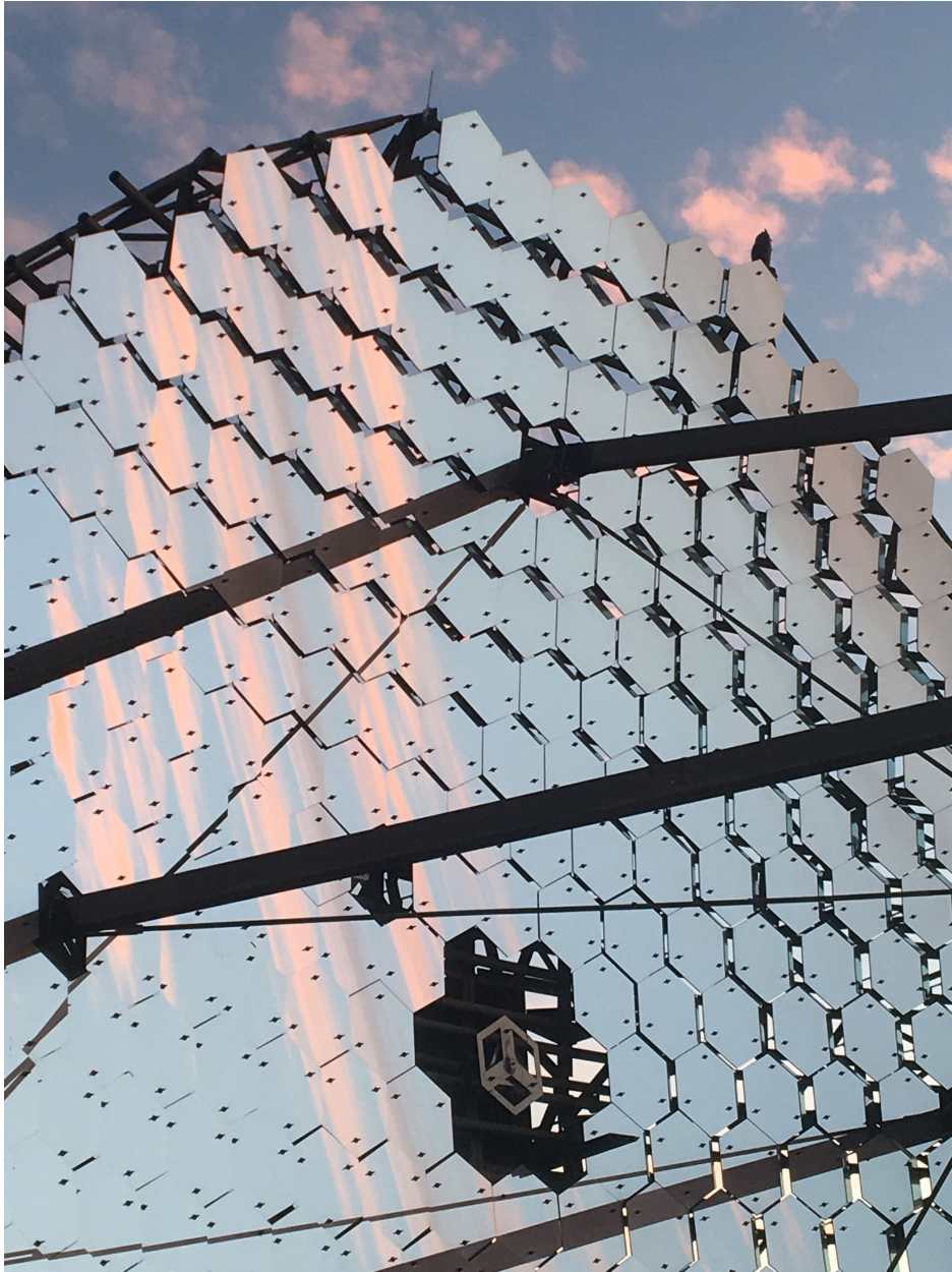
Figure 5.2: A close up of the hexagonal VERITAS mirrors. Each is mounted on three adjustable mounts which allow for manual mirror alignment.
