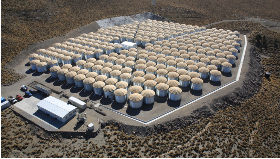
Figure 1.5: The HAWC Gamma-Ray Observatory site near Puebla, Mexico. Visible are the array of 300 water tanks.
