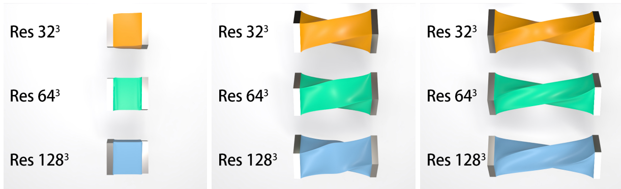
Figure 6.7: Different Mesh Resolution. PBNG produces consistent results when the mesh is spatially refined. The highest resolution mesh in this comparison has over 2M vertices and only requires 40 iterations to produce visually plausible results.
