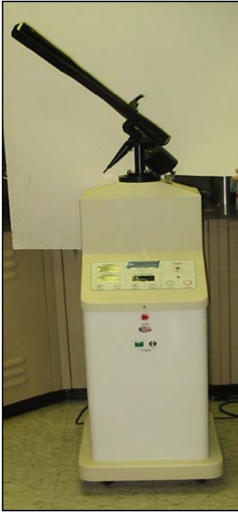
CO 2 laser, Pulse Systems, Inc. (PSI) (Model #LPS-500, Los Alamos, New Mexico)
