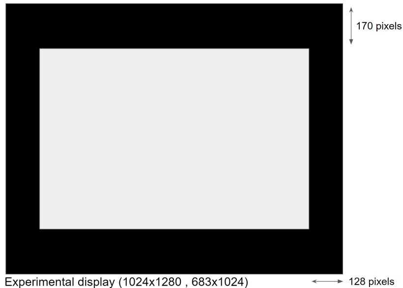
Figure 3.6: Psychophysics 2: Experiment screen for the visual search experiment. The screen is of size 1024 x 1280 with black pixels, and the image of size 683 x 1024 is placed at the center of the screen, shown with gray pixels for illustration.
