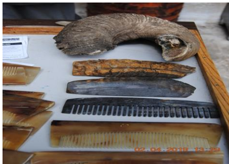
Photo 8: Transformation of the horn into a comb
