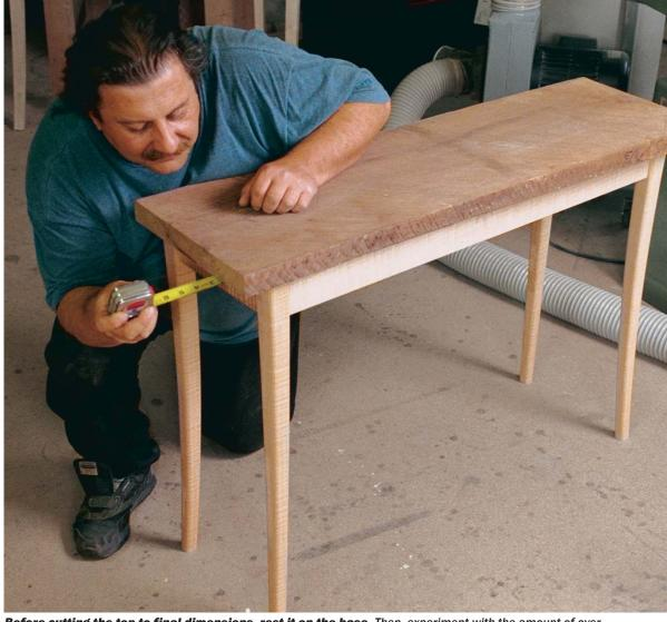
**Before cutting the top to final dimensions, rest it on the base.** Then, experiment with the amount of overhang that looks right to you. The author settled on an overhang of  $\frac{7}{8}$  in. The edge is also beveled under 15°.
