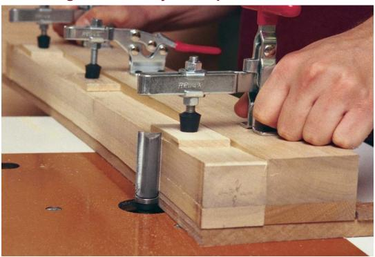
**An easy way to machine the leg.** You can remove all of the waste in one pass with an extralong pattern-cutting bit in an inverted router.
