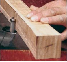
**Use standard bits to machine the leg.** With a 1½-in.-long pattern-cutting bit, you can machine the leg on a router table. First, make one pass with the leg clamped in the jig. Next, remove the leg from the jig and make a second pass, using the machined surface to register the bearing. Finish by using a flush-trimming bit, registering the bearing against an already machined surface.
