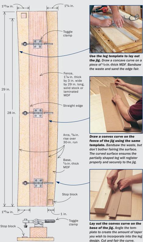
leg. To cut down on steps, use an extralong pattern-cutting bit (see Sources on p. 71) that will allow you to cut each face in one pass (see the bottom photo on the facing page). You still may need to cut each face in two passes because some routers won't let you raise the collet close enough to the throat of the table.
