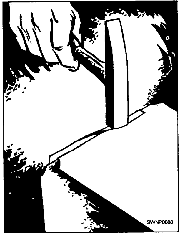
Figure 2-71.—Closing a Pittsburgh lock seam
