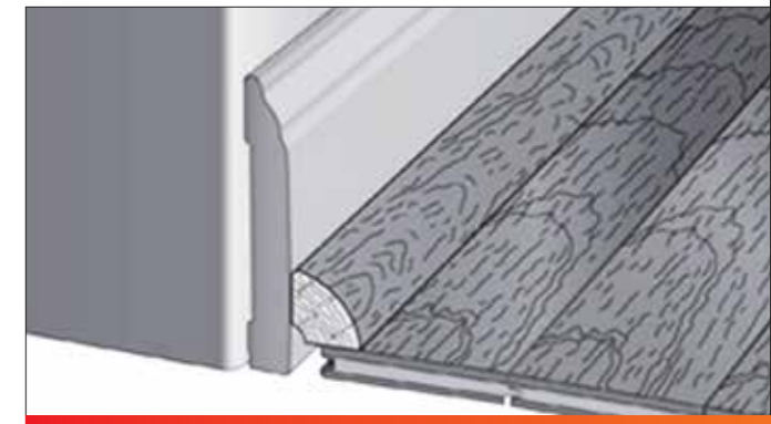
PROFILE USAGE - BEADING PROFILE (cross - sectional view ref Fig No. 11 sheet A)
