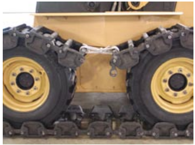
8: Drive the skid steer backwards to position both ends of the track between the tires of the skid steer.
