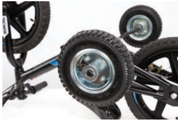
8" Wheel, Washer and Cotter Key Assembled.
