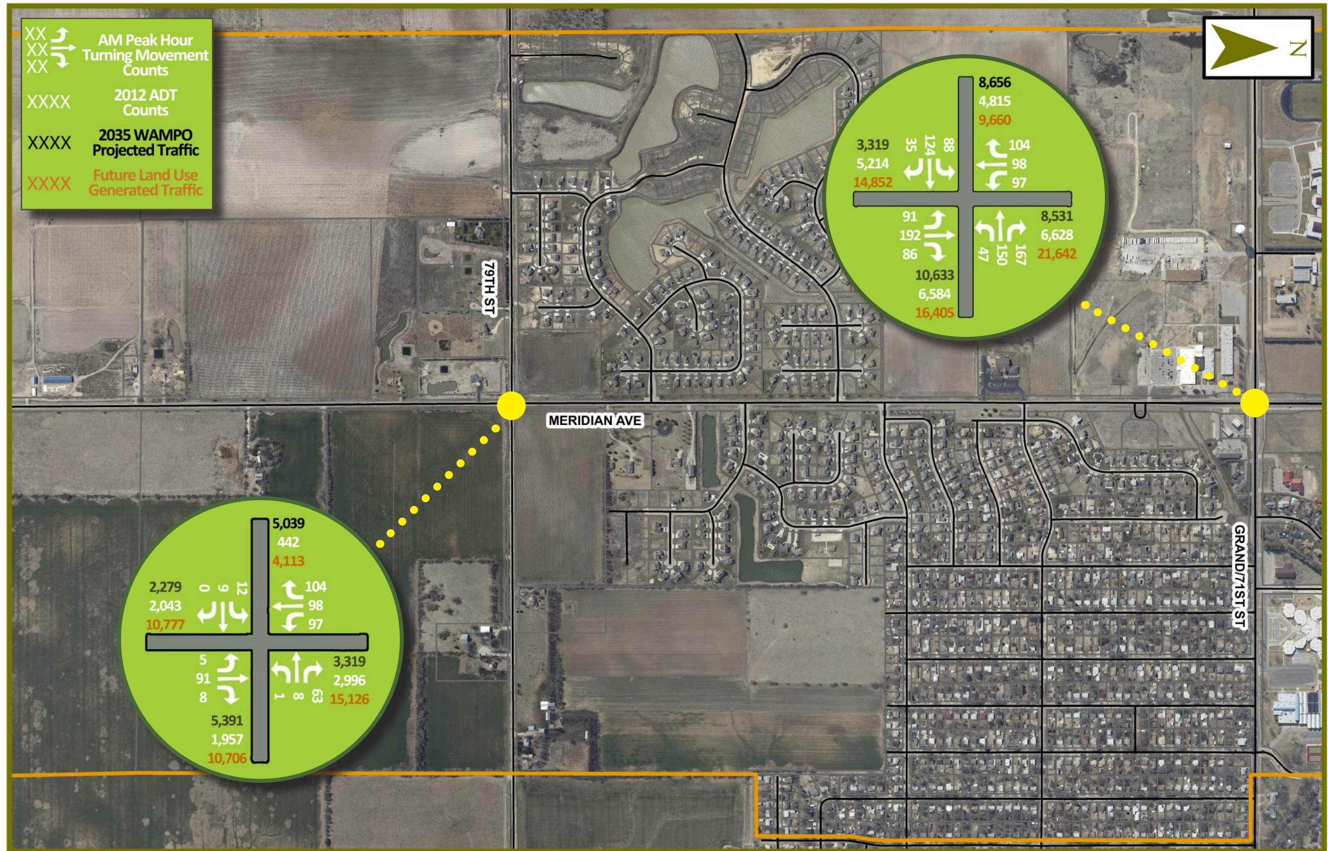
Figure 15: Meridian Traffic Volumes - Center Section
