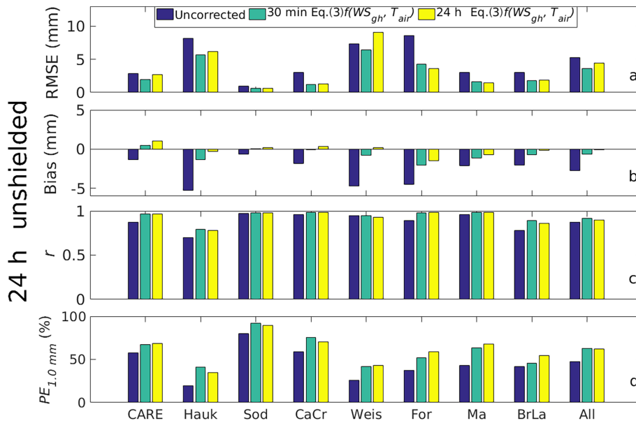
Figure 12. Error statistics for 24h unshielded precipitation measurements that are uncorrected (blue), corrected using the 30 min derived transfer functions (green), and corrected using the 12 h derived transfer functions (yellow) are compared.
