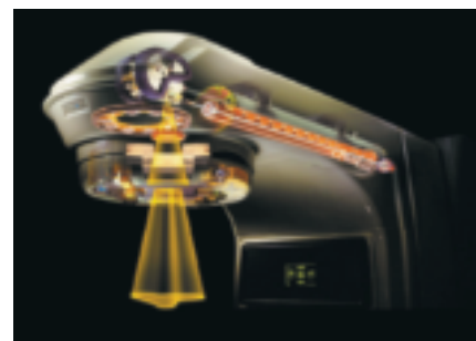
Fig. 6.6 Schematic drawing of the inside of a linear accelerator, indicating the wave-guide in which electrons are accelerated before hitting a target. ©Varian Medical Systems.
