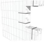
Launching this summer, Alleguard's AmBuck insulated window and door block-out system are stayin-place buck formwork manufactured using Type II/ Type 2 closed cell, Expanded Polystyrene (EPS) panels for ICF construction walls. AmBuck insulated block-out system eliminates the
