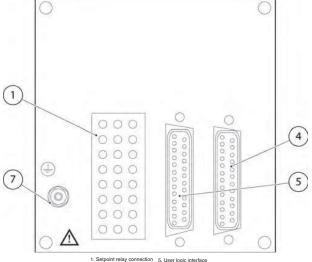
Tic logic interface connection 7. Earth stud
