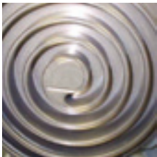
Gas enters scroll set Gas is displaced and... ...compressed toward center hub Gas exhausted at center hub
