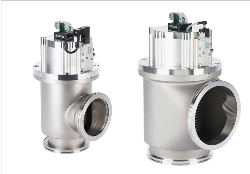
Electropneumatically actuated right-angle valves, bellows sealed, stainless steel, DN 100 ISO-K (left), aluminum DN 160 ISO-K (right)
