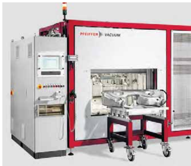
Leak detection system
