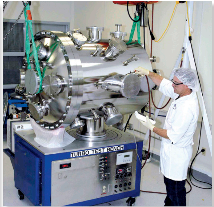
Large Chamber leak testing after mechanical inspection on chamber qualification test bench
