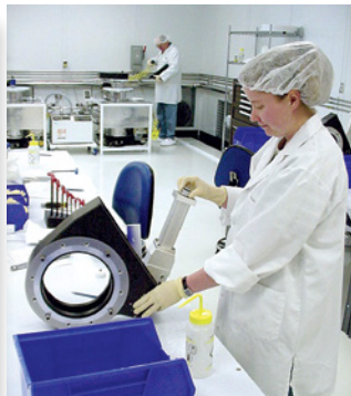
Valve assembly in Class 1000 Clean Room
