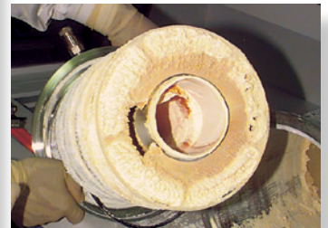
Water-cooled / particle trap for CVD
