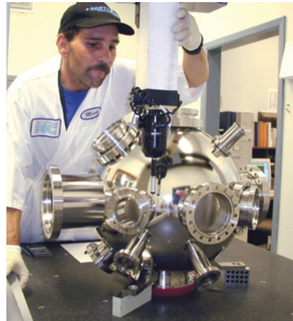
Manual CMM (coordinate measurement machine) inspection
