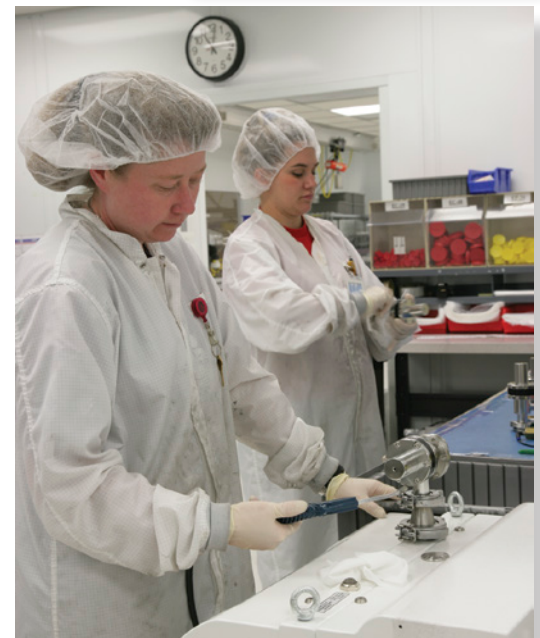
Dry leak detector for valve inspection
