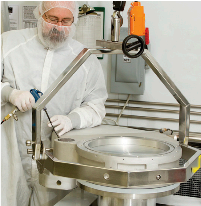
Pendulum valve leak testing in Class 1000 clean room
