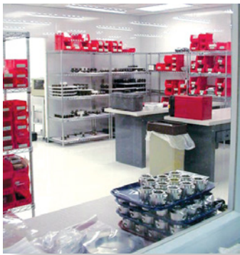
Clean room storage of valve subassemblies
