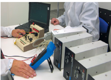
Calibration of Intellisys adaptive pressure controllers
