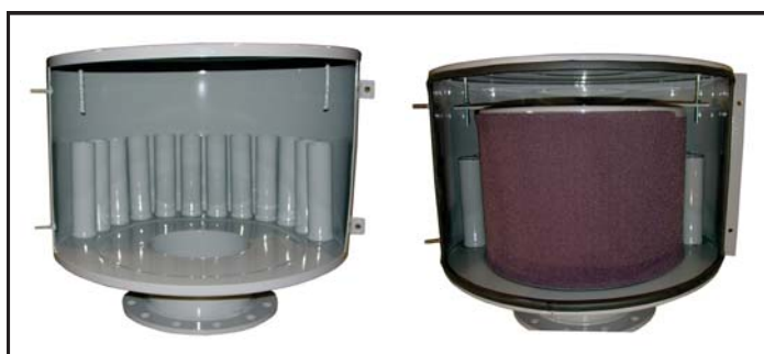
Examples of LQB Silencer Filter with and without filter element installed. Filter element easily slides out the side port for servicing.
