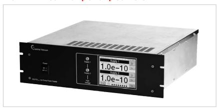
lon pumps 100 l/s and larger required higher currents for starting and higher pressure operation. The QPCe supplies up to four ion pumps with 125 mA (125 watts) each. The easy-to-read color touchscreen display simultaneously displays pressure, current, and voltage. Standard serial and standard Ethernet communications along with legacy setpoint and analog outputs allow for easy system integration. The QPCe fits into any rack at just 3U high and 1/2 rack wide.
