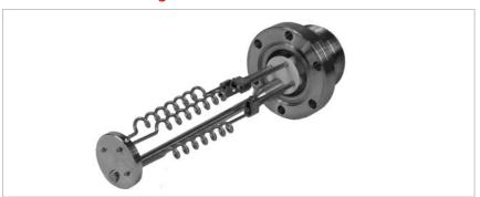
The filament cartridge is mounted on a 2-3/4" CFF (NW 35). The feedthrough supports three titanium-molybdenum filaments and a return path for ground isolation. Each filament contains 1.5 grams of usable titanium and averages 20 hours of operation.
