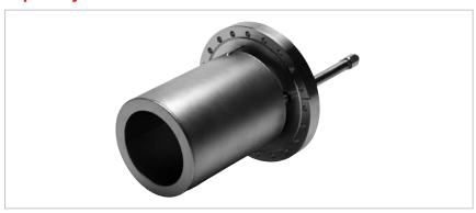
The liquid cryoshroud consists of a double walled, type 304L stainless steel cylinder with two liquid nitrogen feedthroughs with flare type fittings. It provides 1578 cm² (245 in.²) of liquid nitrogen cooled surface area that provides pumping speeds up to 12,000 l/s for hydrogen (see table). The shroud is mounted on an 8 in. CFF (DN 160) or 10 in. CFF (DN 200)
