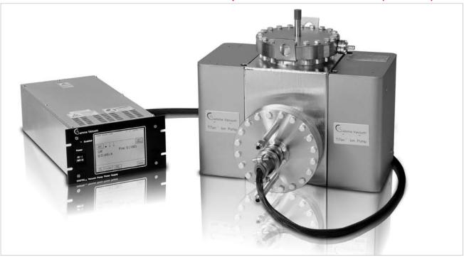
Titanium Sublimation Pumps (TSPs) are often used in combination with ion pumps or independently to remove reactive gases from the vacuum environment. Combined with an ion pump, the TSP allows for low ultimate pressures in a shorter amount of time. All TSP components are bakeable to 400°C.
