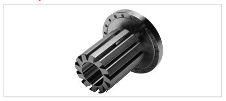
The ambient sputter shield economically maximizes surface area when cooling is not practical or possible. It provides 827cm2 (128 in.2) of ambient temperature surface area that provides pumping speeds up to 2,200 l/s for hydrogen (see table). The shield is mounted on an 8 in. CFF (DN 160) or a 6 in. CFF (DN 100).
