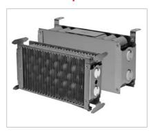
TiTan™ ion pump elements are "tuned" for specific pumping applications. Surfaces are chemically processed to remove potential surface contaminants and provide maximum adhesion for extended lifetime. Ceramics are optimally shielded to reduce exposure to sputtered material.
