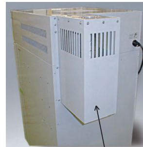
Sample oven with exhaust duct
