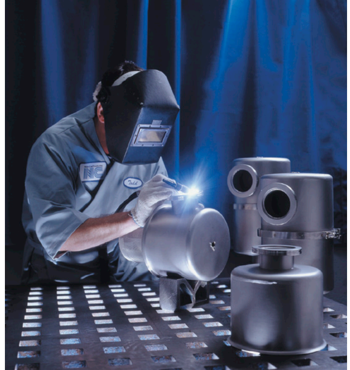
TIG Fusion Welding
