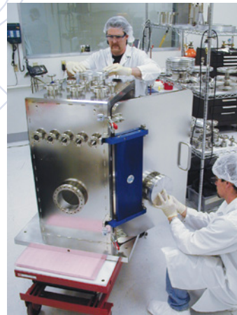
High vacuum chamber used to house an X-ray scanner in the Sandia National Laboratory LIGA project
