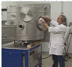
Vacuum coating chamber
