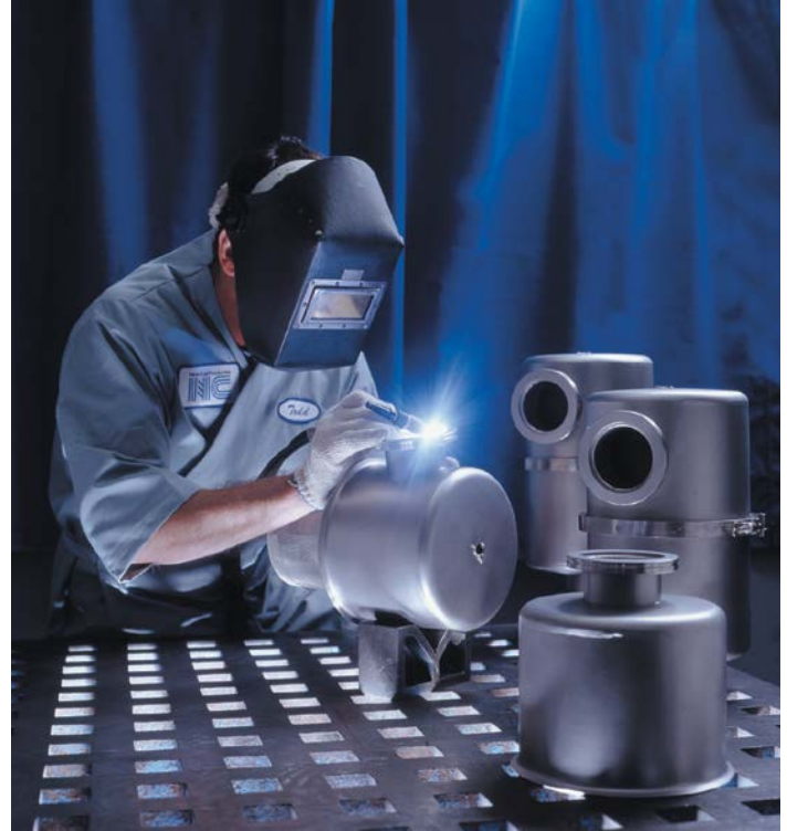
TIG Fusion Welding
